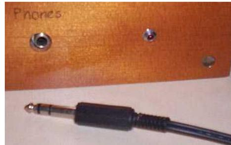
Fig 2: 6.5mm plug & socket
