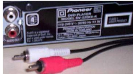
Fig 1: RCA type plugs & sockets
