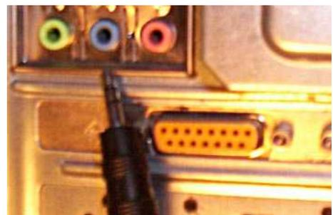
Fig 4: Connecting to the 'Line In' socket on the PC
