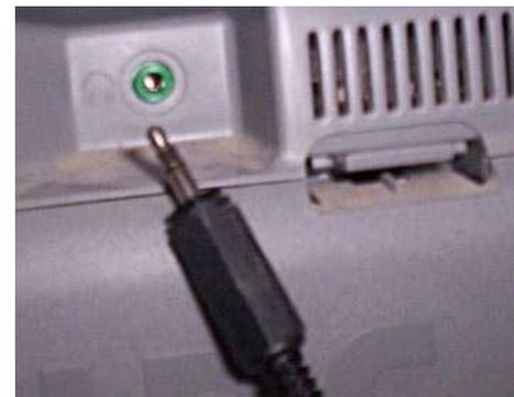
Fig 3: 3.5mm plug & socket
